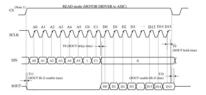
Note 1) CS default value of each cycle (Write / Read mode) starts from Low-level. Note 2) It is necessary to input the system clock OSCIN at write mode.
