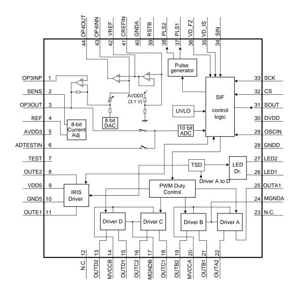
Note) This block diagram is for explaining functions. The part of the block diagram may be omitted, or it may be simplified.
